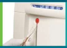
Due to its automatic retractable and self-wiping fill port, can aspirate whole blood, serum, urine, or other biological substance from syringe, tube or capillary, from 40uL for 2 electrolytes.
