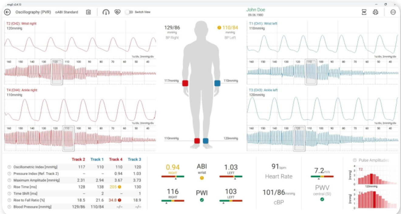
4-Channel simultaneous Pulse Wave Recording on Arms and Ankles.
