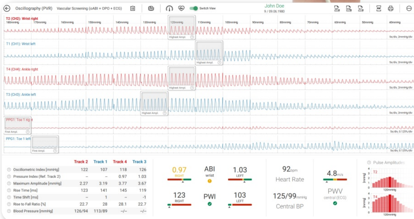
6-Channel Simultaneous Pulse Wave Recording on Wrists, Ankles and Toes using the TOPP-Method (Tissue Optical Perfusion Pressure).
